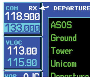
Press the COM power/volume knob momentarily to override the automatic squelch. Note the "RX" receive indication when receiving a station.
