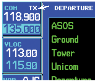
"TX" appears at the upper right corner of the COM window while transmitting.
