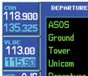
Cursor in VLOC window allows for VOR and ILS operations.
